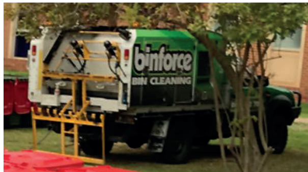
Figure 4.4 On-site bin wash system for rear-lift trucks on back of ute. Source: http://binforce.com.au/
