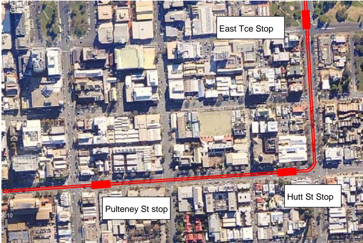
Two way non-dedicated light rail line (within traffic lane) on Hutt Street. It is not intended that stops be located on Hutt Street, as this would disrupt the flow of traffic.
